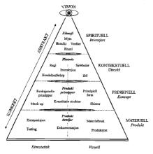
Erik Lerdahl introduces a model for work on different levels of abstraction in the design process: visionary, spiritual, contextual, principle, material. The process can move freely between all levels during the whole process.
